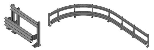
Figure 7. Bridge side guardrail modeling results using Revit "railing" family.
