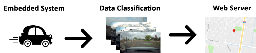
Figure 1. Overview of the proposed system; the embedded system mounted on a volunteers car will capture images while driving normally; then, the system will process the images in real time and send data to a remote server only if the image contains at least one of our proposed classes; the server will then save the image and location of said class.
