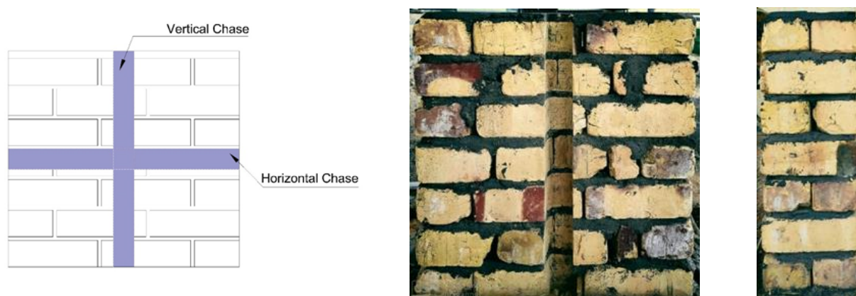
Figure 4. Creation of the vertical and horizontal chases.
