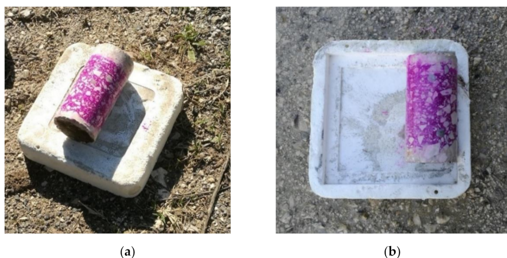
Figure 7. Samples B1_1 (a) and B1_2 (b) after phenolphthalein spraying.
