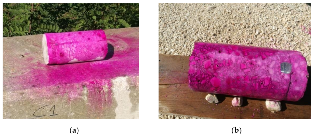
Figure 6. Samples C1 (a) and C2 (b) after phenolphthalein spraying.
