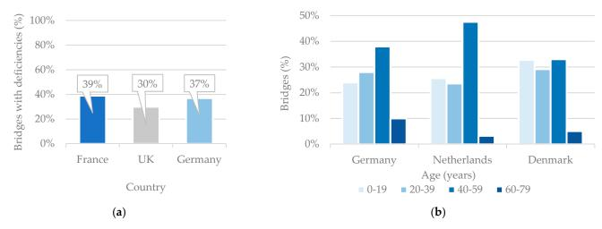
**Figure 1.** (a) Estimated percentage of highway bridges with deficiencies (adapted from [2]); (b): age of bridges in Germany, the Netherlands, and Denmark over the Trans-European Transport Network (TEN-T) (adapted from [3]).
