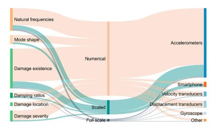
**Figure 2.** Interconnection between scope (structural modal identification and damage detection), publication type, and sensing units.
