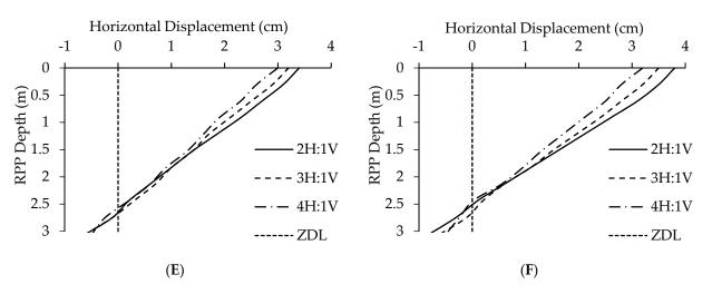
**Figure 6.** Horizontal displacement profile of RPPs at the crest of the highway slopes: (**A**) configuration A, (**B**) configuration B, (**C**) configuration C, (**D**) configuration D, (**E**) configuration E, and (**F**) configuration F (Zero Displacement Line (ZDL)).
