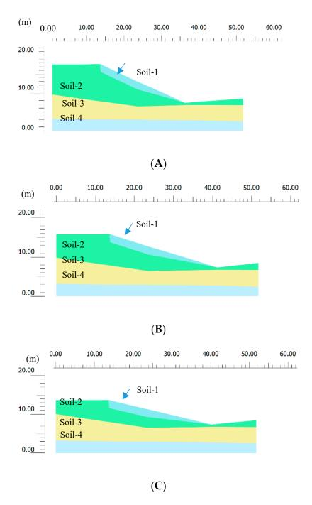
Figure 2. Slope geometries for (A) 2H:1V slope, (B) 3H:1V slope, and (C) 4H:1V slope.
