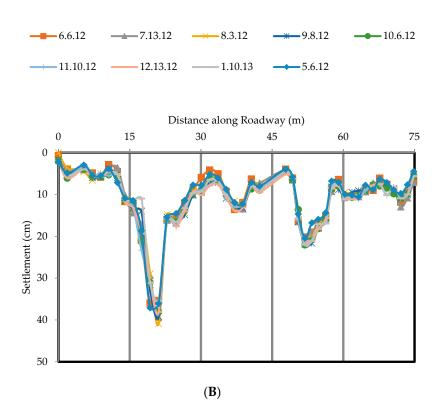
**Figure 1.** Performance of US 287 slope (**A**) the layout of RPP and (**B**) total settlement profile at the crest of the slope [11].
