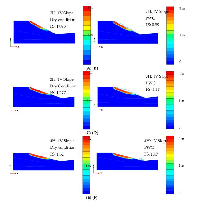
**Figure 3.** Stability analysis of the unreinforced slope: (**A**) 2H:1V slope (dry condition), (**B**) 2H:1V slope (PWC), (**C**) 3H:1V slope (dry condition), (**D**) 3H:1V slope (PWC), (**E**) 4H:1V slope (dry condition), and (**F**) 4H:1V slope (PWC).
