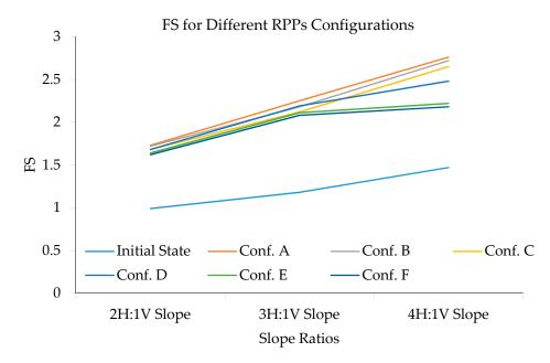
**Figure 5.** Variations in the FS for different RPP configurations for the three slope ratios of 2H:1V, 3H:1V, and 4H:1V.
