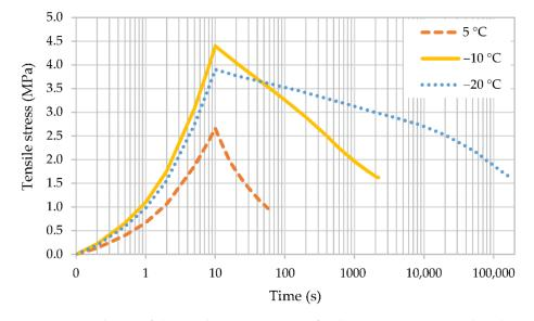
**Figure 10.** Evolution of the tensile stress over time for the PMB25 mixture in the relaxation test at different temperatures.
