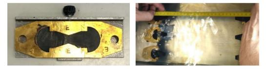
Figure 1. Elastic recovery test of polymer-modified binders: molds and measuring procedure.
