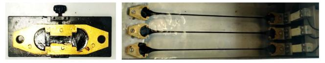
Figure 2. Force ductility test of PMBs: molds and specimens elongated.
