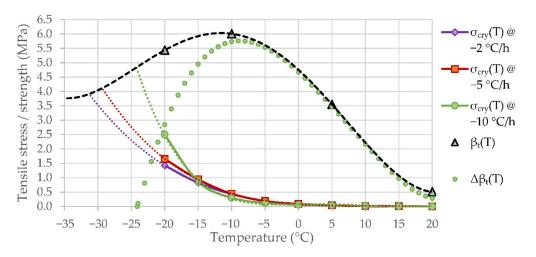
**Figure 9.** Mean results of the thermal stress restrained specimen test (TSRST) tests for PMB25 mixture at three different cooling rates.
