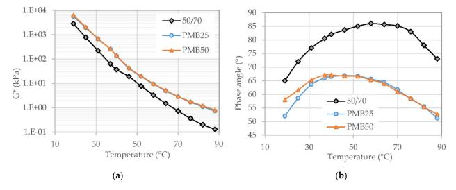
**Figure 5.** Rheological characteristics of the asphalt binders, i.e., the base bitumen 50/70, PMB with 2.5% SBS (PMB25), and PMB with 5.0% SBS (PMB50): (**a**) Complex shear modulus ( $G^*$ ); (**b**) phase angle ( $\delta$ ).
