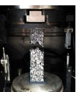
Figure 7. Example of tested specimen in the UTST test.
