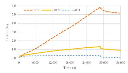
Figure 11. Results of tensile creep tests on the PMB25 mixture at different temperatures.
