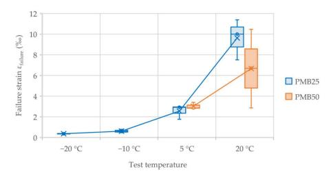
**Figure 8.** Failure strain results,  $\varepsilon_{\text{failure}}$ , from the uniaxial tension stress test (UTST) for SMA 11 mixtures with PMB25 and PMB50.
