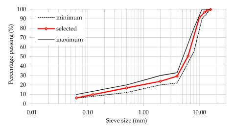
**Figure 4.** Selected grading composition curve for stone mastic asphalt with a maximum aggregate size of around 11 mm (i.e., SMA 11) mixtures.
