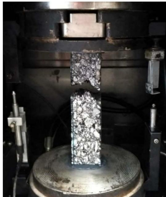
Figure 7. Example of tested specimen in the UTST test.
