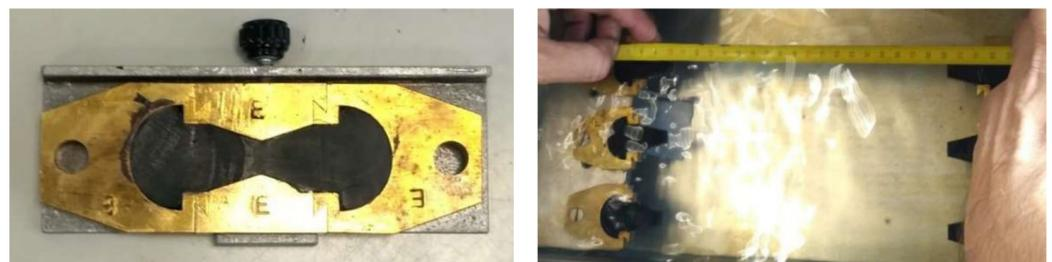
**Figure 1.** Elastic recovery test of polymer-modified binders: molds and measuring procedure.
