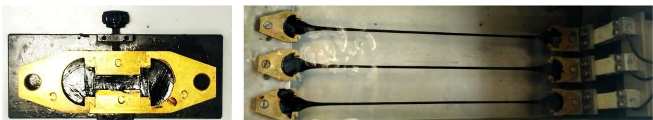
**Figure 2.** Force ductility test of PMBs: molds and specimens elongated.
