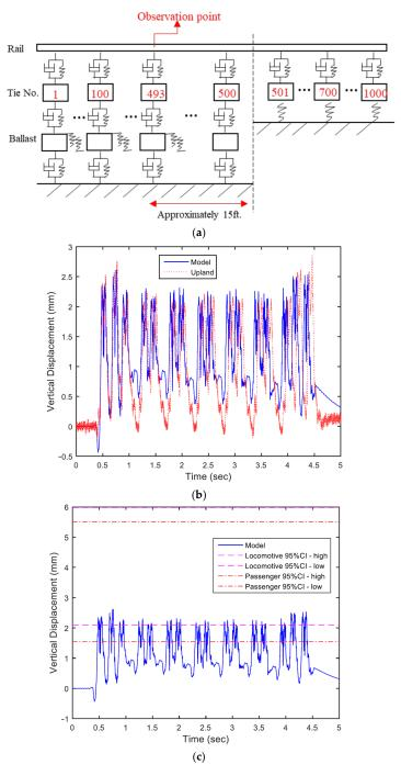
**Figure 10.** Near Bridge Location: (a) Sketch of the response observation point in the model; and (b) comparisons of model predictions and field data.
