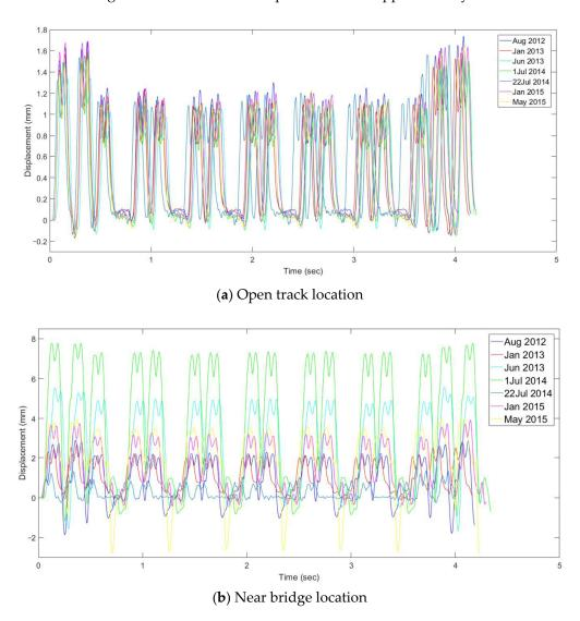
Figure 4. Transient vertical deformations with train passage at Upland.
