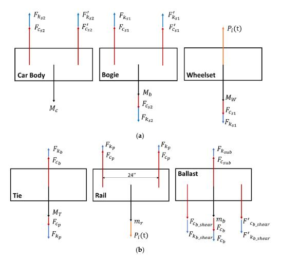
Figure 7. Free Body Diagrams for (a) vehicle components and (b) track components.
