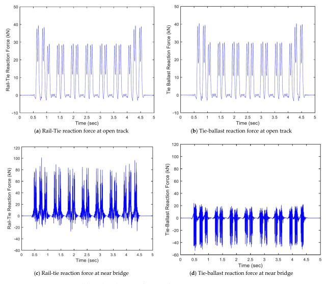
Figure 11. Model predicted reaction forces with ACELA Express passenger train passage.
