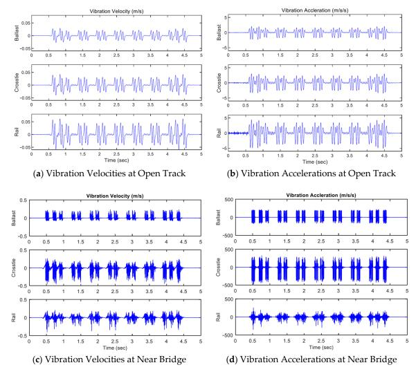
Figure 12. Model predicted structural vibration velocities and accelerations with ACELA Express passenger train passage.
