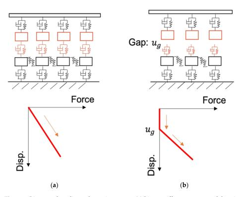
**Figure 8.** Linear and nonlinear dynamic systems: (a) Linear stiffness at open track location, and (b) nonlinear stiffness at near bridge location.
