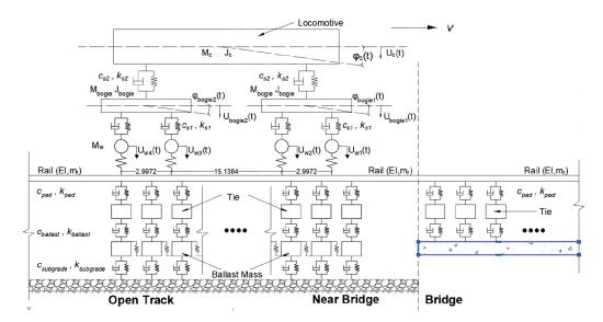
Figure 6. Train-Track-Bridge Model developed at the University of Illinois.
