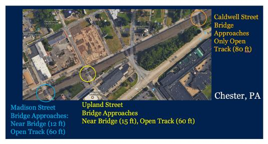
**Figure 1.** Locations of the Three Bridges Selected for Instrumentation in Amtrak's NEC (1 ft = 30.5 cm).
