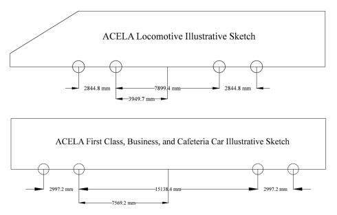
Figure 3. ACELA locomotive and passenger car axle spacings.
