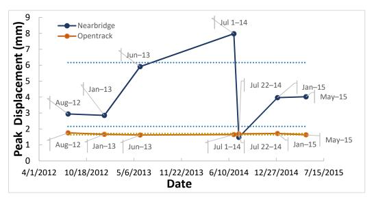
Figure 5. Upland peak vertical transient deformations over time (2012–2015).
