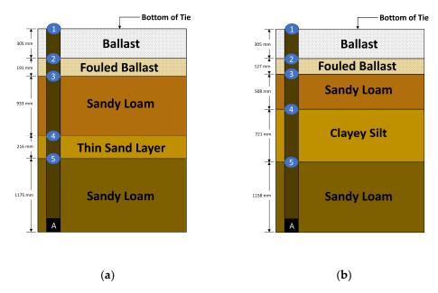
**Figure 2.** Substructure Layer Profile for (a) Upland Street 4.6 m (15 ft.) from the North Abutment; and (b) Upland Street 18.3 m (60 ft.) from the North Abutment.
