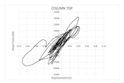
Figure 8. Displacement vs. shear force at the top of the column for the most severe earthquake.
