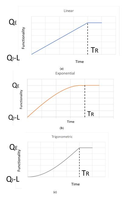
Figure 1. (a) Recovery model (linear); (b) recovery model (exponential); (c) recovery model (trigonometric).
