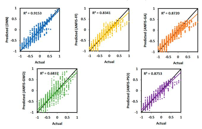
**Figure 8.** Illustration of actual and predicted strain in lateral (*x*) dimension (Training phase).
