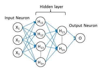
Figure 2. Architecture of a deep neural network (DNN) for strain prediction.
