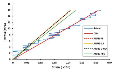
**Figure 6.** Stress-Strain behavior of rock sample (*x* direction).
