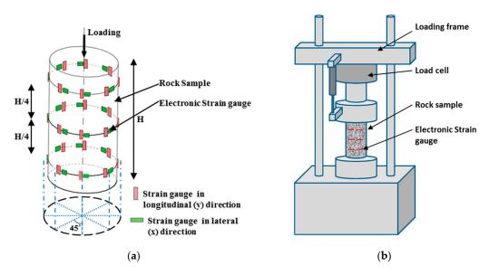
**Figure 1.** (a) Details of strain gauge location with uniaxial load of rock sample and (b) Experimental Setup.
