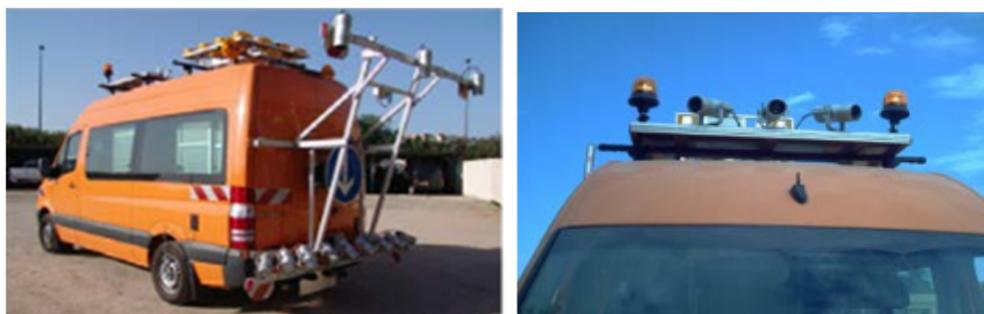
**Figure 1.** Multifunctional Pavement Inspection System SMAC with macro cameras (left) and front cameras (right).
