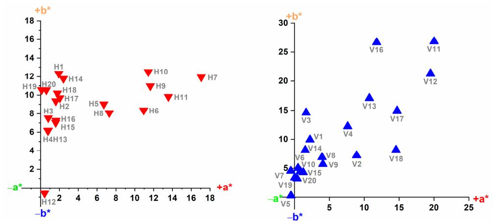
Figure 6. Color coordinates a\* and b\* of the materials analyzed in situ. **Left:** horizontal surface finishes. **Right:** vertical surface finishes.
