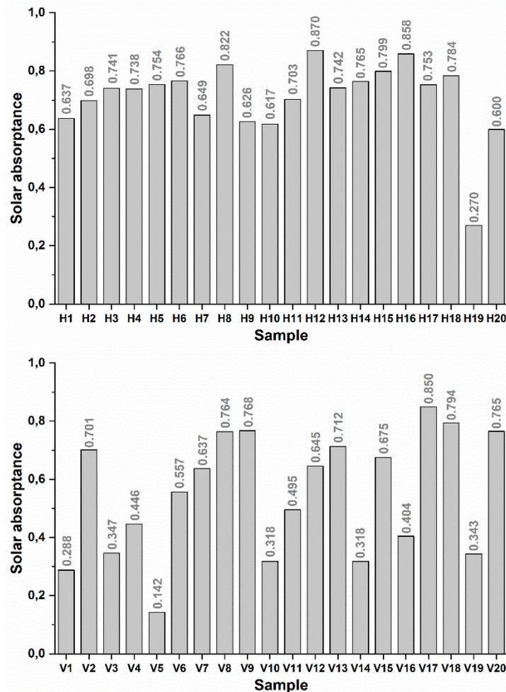
Figure 4. Solar absorptance of the materials analyzed in situ. Top: horizontal surface finishes. Bottom: vertical surface finishes.
