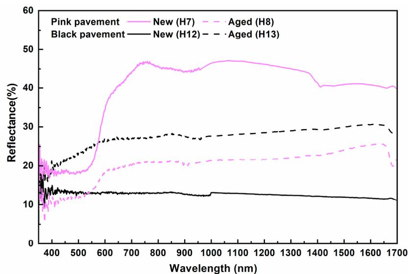
Figure 7. Mean reflectance spectra of the different horizontal surface finishes shown in Figure 2.
