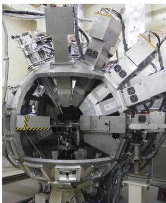
**Figure 20.** Diffractometer of iBIX.
