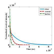
**Figure 2.** The impulse responses for three types of water: clear (50 m), coastal (20 m) and harbor (4 m).
