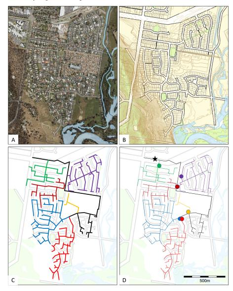
**Figure 2.** Conceptual example of retrofitting stratified sampling points to an existing development in Albury, NSW, Australia. (**A**) Aerial image; (**B**) street and contour map; (**C**) existing sewerage net-work color coded to show subnetworks; (**D**) suggested interception and sampling points (aerial photograph, base map and sewer alignment based on data derived from the Albury City Mapping Portal).
