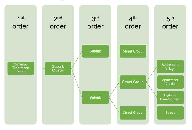
Figure 1. Conceptual example of hierarchical clustering of sampling points.
