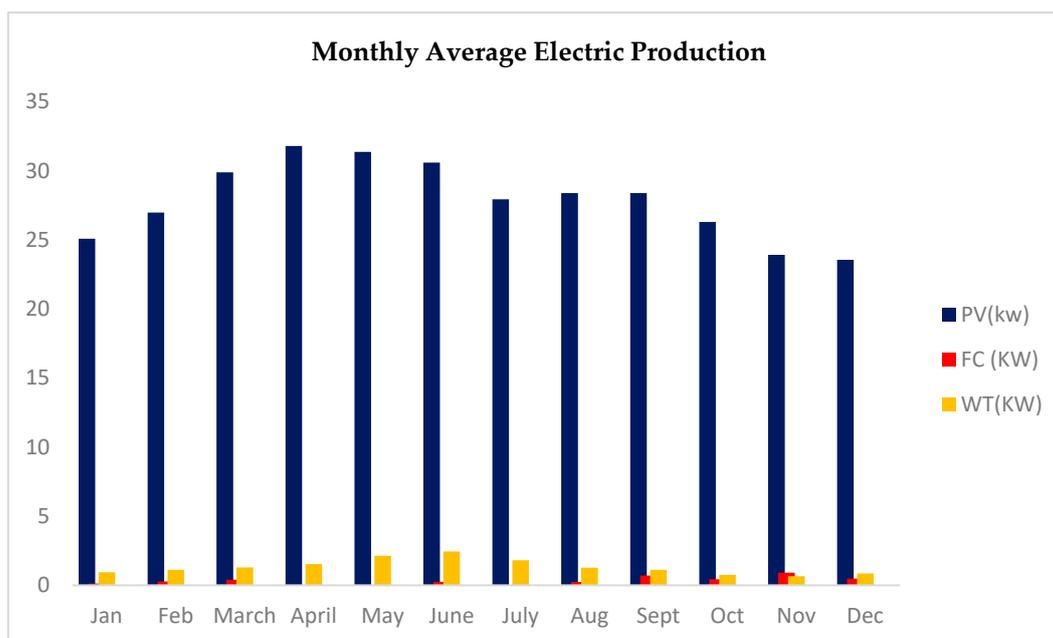
**Figure 7.** Estimated monthly electricity produced by each component of the off-grid hybrid system.**Table 5.** Pricing description of the ideal hybrid off-grid energy systems.
