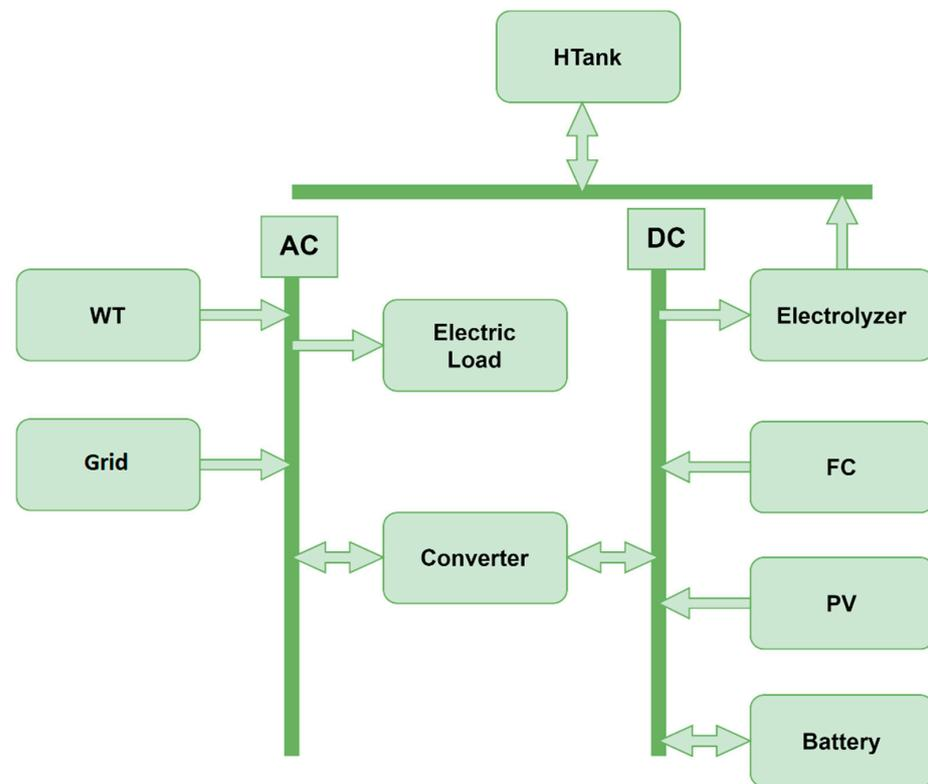
**Figure 5.** A generalized design of a grid-connected, wind-solar, and fuel-cell power system including backup batteries and a hydrogen tank.
