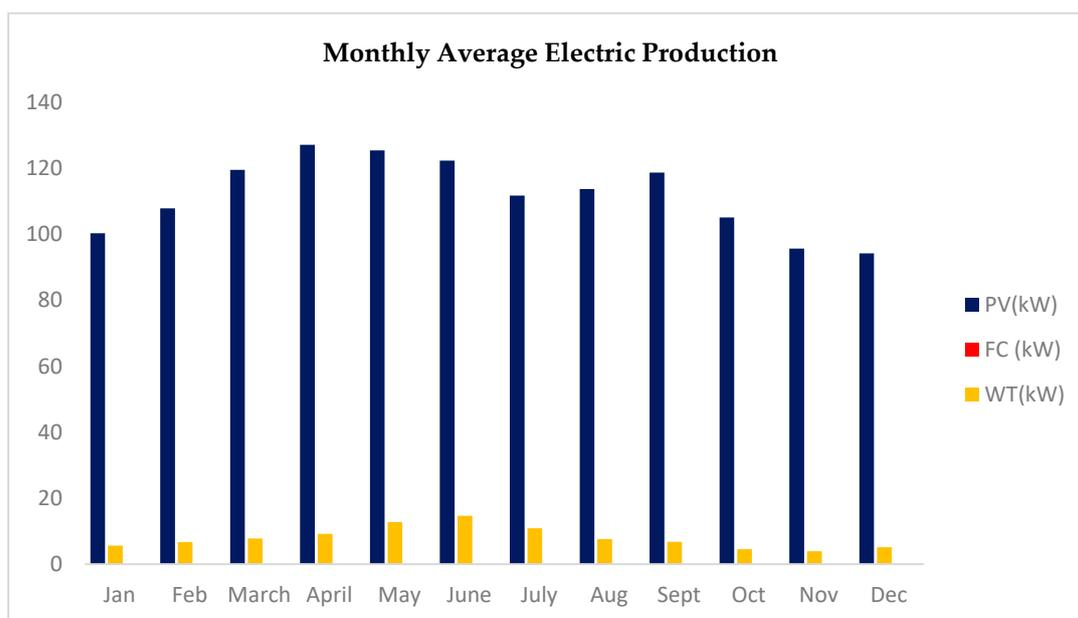
**Figure 8.** Estimated monthly electricity produced by each component of the grid-connected hybrid system.
