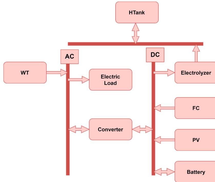
**Figure 4.** A generalized design of a wind, solar, and fuel-cell power system including backup batteries and a hydrogen tank.
