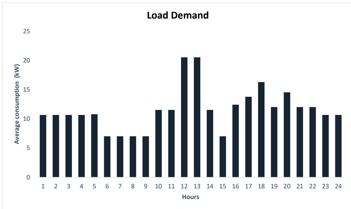
**Figure 3.** The required remote area electrical demand.
