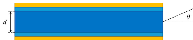
Figure 3. Geometry of the end of the sensor (Au-coated fibre): d = fibre core diameter; \theta = maximum acceptance half-angle.
