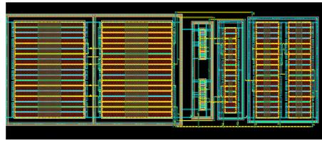
**Figure 15.** Layout of the CMOS OTA providing  $g_m = 500 \mu\text{A/V}$ .
