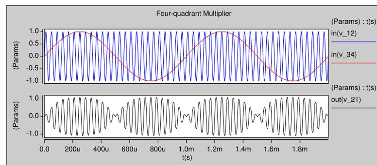
Figure 12. Multiplication of two signals using the CMOS design from Figure 11.
