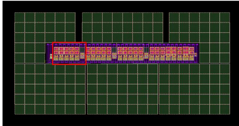
Figure 20. Layout of our proposed CMOS OTA-based  $\text{FOCO}_1$  shown in Figure 6.
