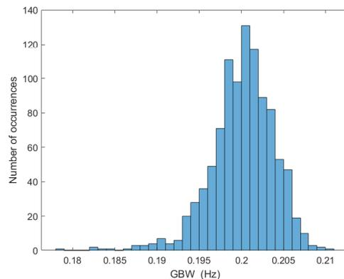
**Figure 19.** Monte Carlo simulation of our proposed CMOS fractional-order integrator shown in Figure 16.
