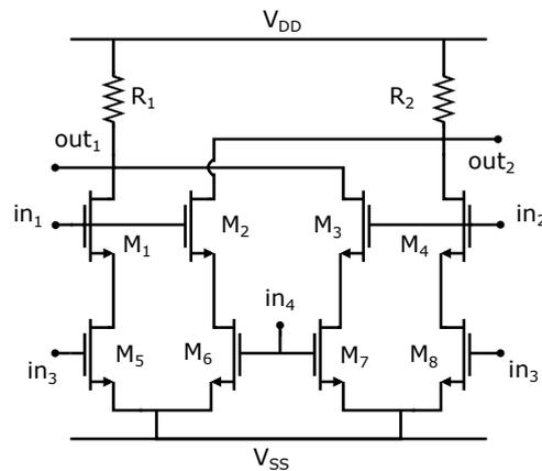
Figure 11. Fully differential four-quadrant multiplier taken from [38].
