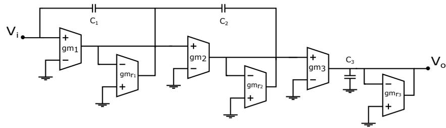
**Figure 5.** Proposed OTA design of  $\frac{1}{s^{0.9}}$  that is approximated by (7), and designed by cascading  $H_1(s)H_2(s)H_3(s)$ .
