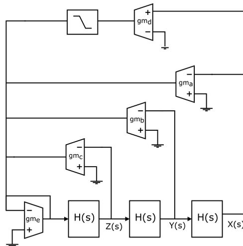
Figure 8. Proposed OTA implementation of the  $\text{FOCO}_2$  given in (5).
