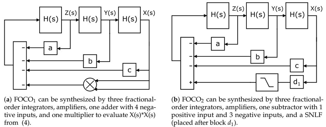
Figure 3. Block diagrams of the FOCOs, where  $H(s) = 1/s^{0.9}$ .
