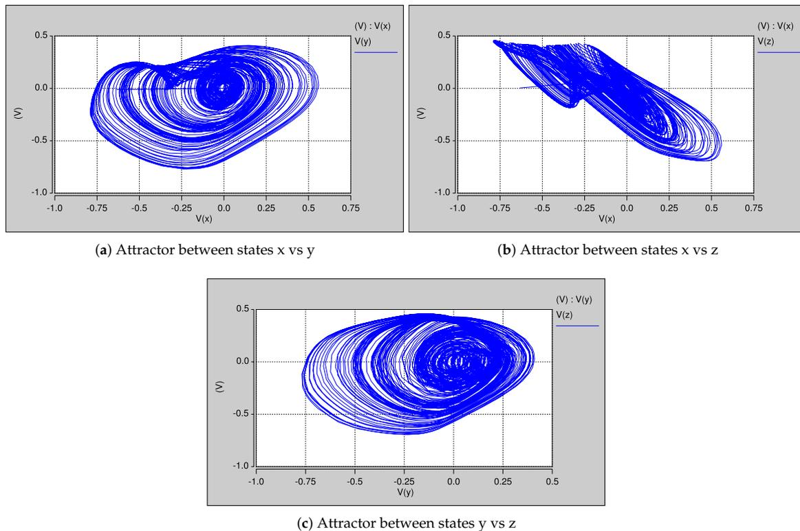
Figure 21. Portraits of the post-layout simulation of our proposed CMOS OTA-based  $\text{FOCO}_1$ .
