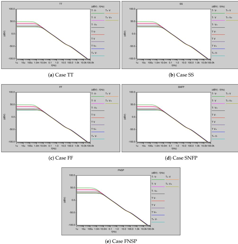
**Figure 18.** Process–voltage–temperature (PVT) variation simulations of the CMOS fractional-order integrator shown in Figure 16.
