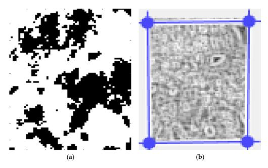
**Figure 26.** Secondary processing of the selected image 3: (a) binarized version; (b) application of the mask. A threshold of 25 was used for binarization.
