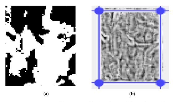
**Figure 17.** Secondary processing of the selected image 2: (a) binarized version; (b) application of the mask. A threshold of 25 was used for binarization.
