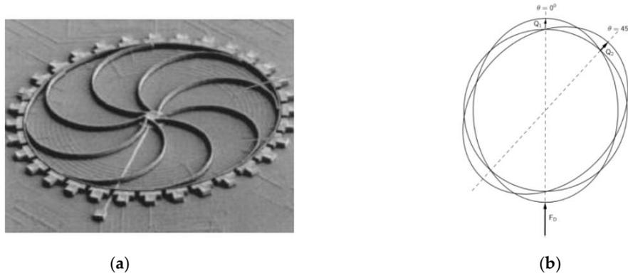
**Figure 1.** (a) Typical configuration for ring-based CVG having 8 support spokes [3]; (b) For devices operating using  $2\theta$  in-plane flexural responses, the drive mode is excited at resonance by applying a harmonic drive force; rotation about the ring polar axis induces the sense mode to vibrate, aligned 45 degrees to the drive mode.
