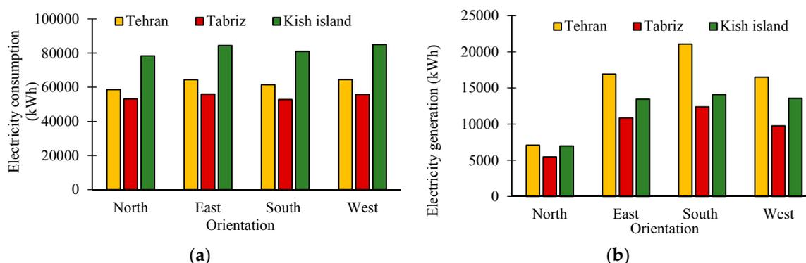
**Figure 1.** Energy performance of the PV-DSF building: (a) energy consumption of the PV-DSF building; (b) electricity generation of the PV-DSF building.
