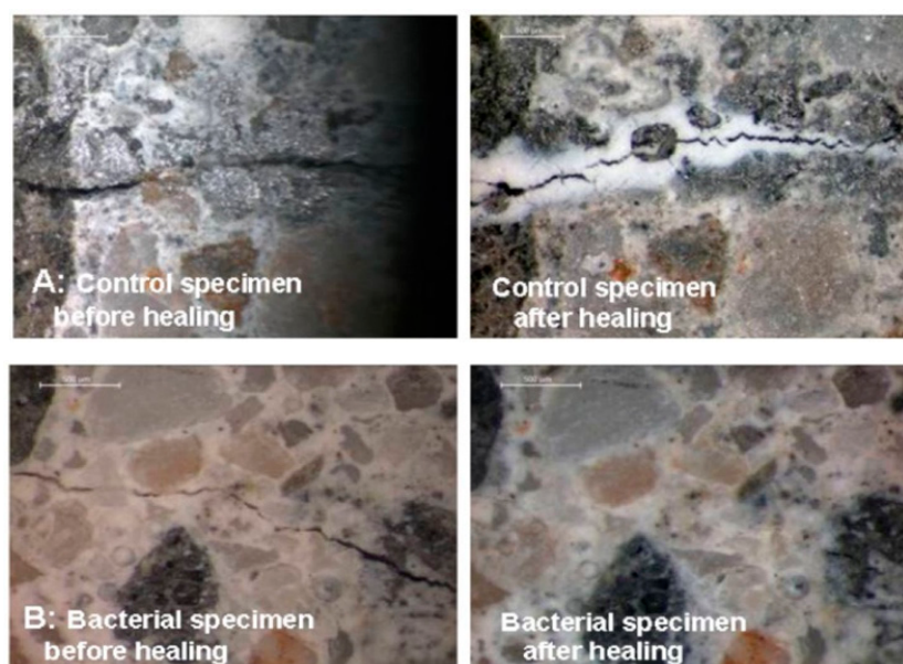
Figure 5. Images of pre-cracked control (A) and bacterial (B) concrete specimen before and after healing [6].
