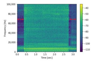
**Figure 7.** A typical spectrogram of one pass. In the dark blue vertical areas, highlighted by the red arrows, the tool is outside of the machining area. The color, in log scale, represents the intensity of the signal.
