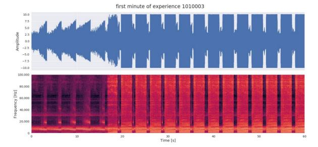
**Figure 6.** Transformation of the signal from the time domain to the related spectrogram. On the left, we can observe that the first 5 passes are outside the material (no-machining), the sixth touches the material only partially, and the following passes characterize the normal machining behavior.
