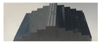
**Figure 5.** This figure shows the details of a workpiece. The left side was machined with a tool at the end of its lifespan. The presence of multiple chips in the material indicates that the quality of the stair edges has deteriorated.
