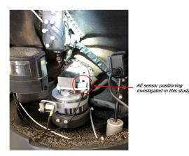
**Figure 2.** Acoustic emission sensor positioning. As highlighted by the red circle, the AE sensor is glued to the material that is being machined.
