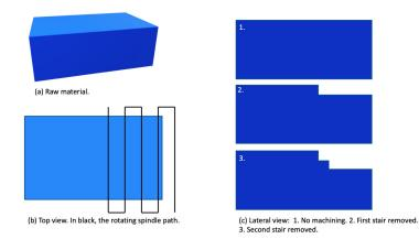
**Figure 3.** A visual representation of the milling operation investigated in this study. (a) The raw material before the machining; (b) in black, from the right to the left, the path of the cutting tool. In the representation, we can observe 5 passes, of which 1 is outside the material, and 4 are in the material–top view. (c) Removal of the first 2 levels of the material-lateral view.
