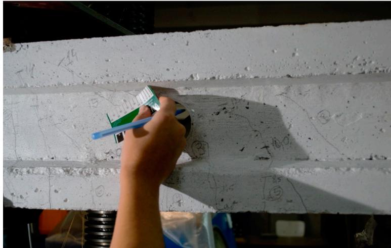
Figure 2. Marking and mapping cracks.
