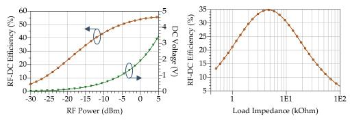
**Figure 5. RF-DC** Power conversion efficiency of the textile rectifier for different RF power levels (left) and load impedances (right).
