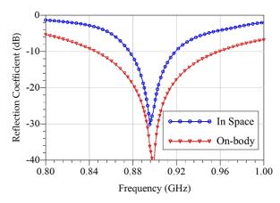
**Figure 3.** Measured return loss of the single-thread monopole, with a large ground plane, showing a 4.6% fractional impedance bandwidth.
