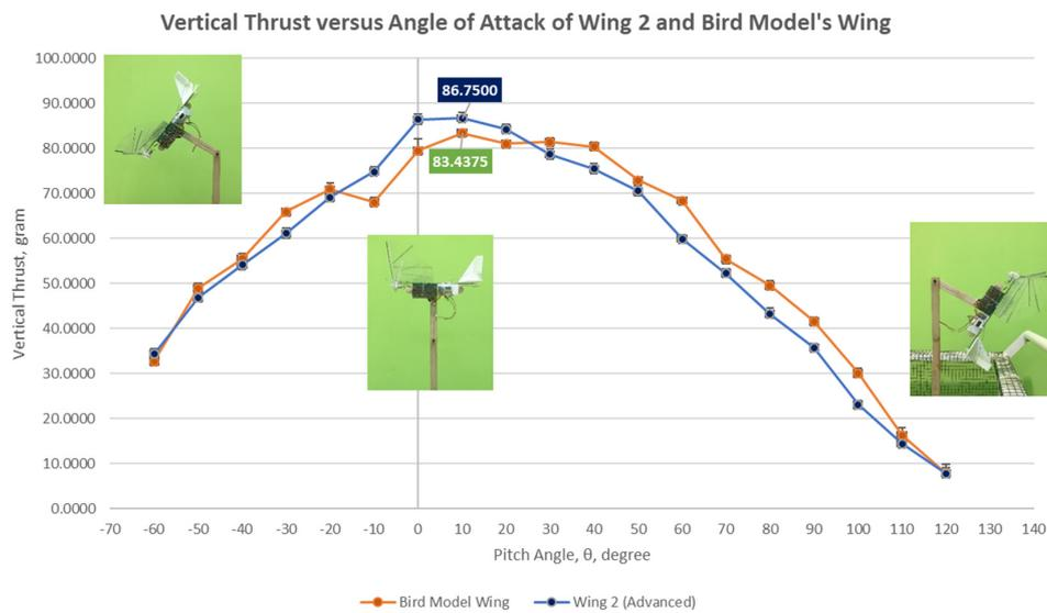
Figure 19. Graph of vertical thrust versus pitch angle for the bird model wing and wing 2.
