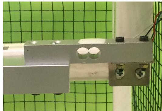
(b) A 5 kg straight bar load cell with HX711 amplifier module
