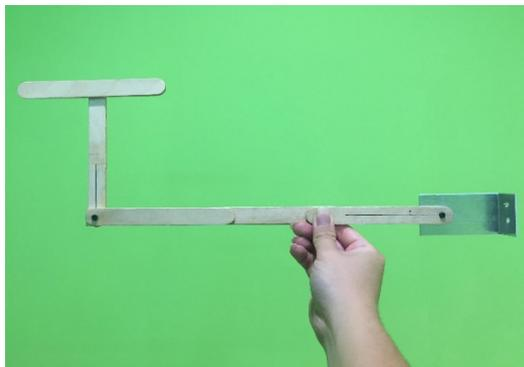
(a) T-shaped jig with a rotating mounting of the FW-MAV
