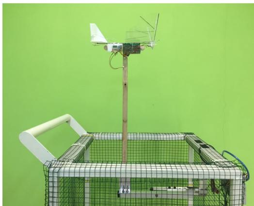
(c) The completed setup of vertical thrust measuring load cell setup
