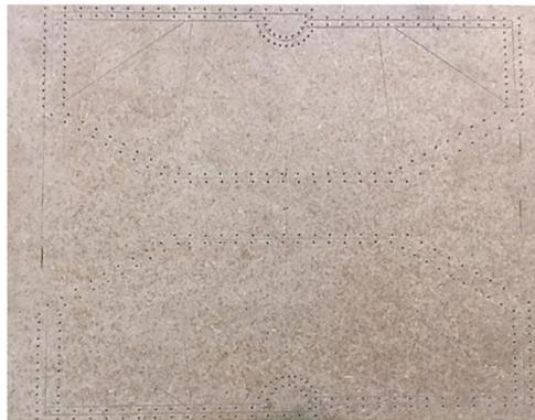
**Figure 6.** The MDF mold after milling and drilling.
