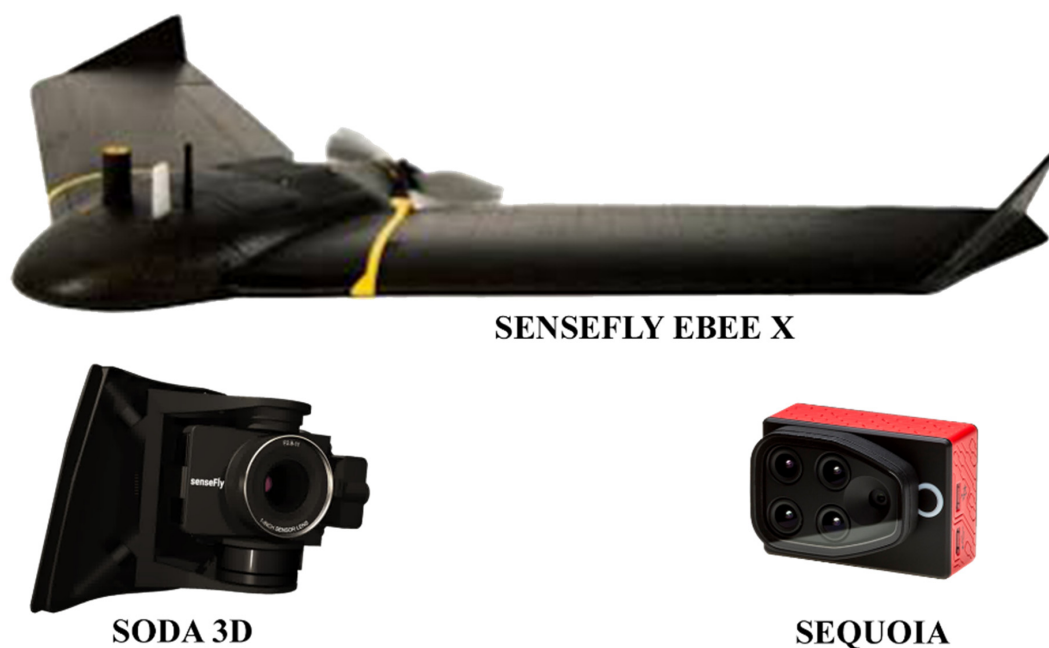
Figure 5. Sensefly fixed-wing eBee Plus with S.O.D.A. 3D and Parrot Sequoia cameras.
