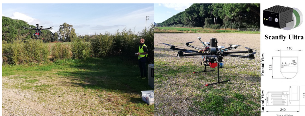
Figure 4. The ScanFly system with LiDAR Velodyne Ultra Puck sensor.
