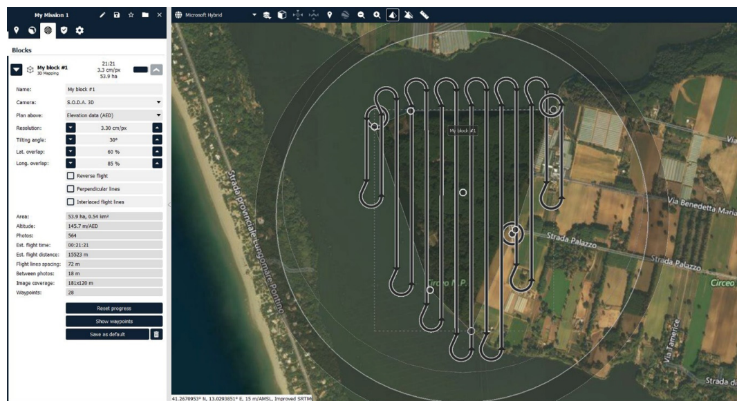
Figure 7. Flight plan in Emotion for RGB image acquisition with Sensefly eBee X.
