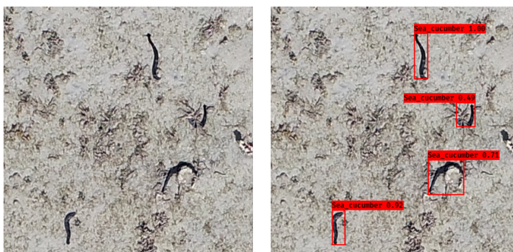
Figure 4. Detection result sample. Left: cropped image before detection. Right: detected results with bounding boxes and detect confidence plotted on each sea cucumber.
