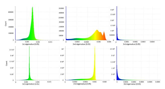
**Figure 7.** Histogram of  $\lambda_1$ ,  $\lambda_2$  and  $\lambda_3$  estimated within a local sphere with a radius 0.05 m from RPAS-based (on the (**top**)) and TLS-based (on the (**bottom**)) point clouds, respectively.
