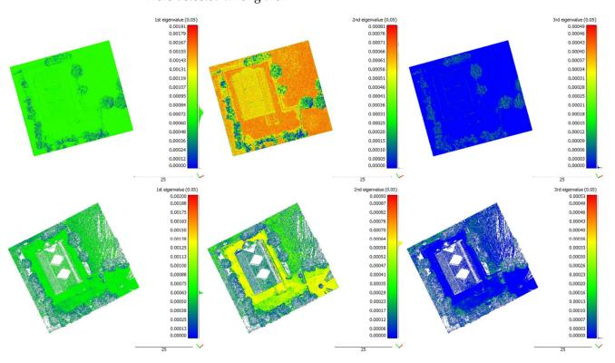
**Figure 6.**  $\lambda_1$ ,  $\lambda_2$  and  $\lambda_3$  estimated within a local sphere with a radius 0.05 m from RPAS-based (on the (**top**)) and TLS-based (on the (**bottom**)) point clouds, respectively.
