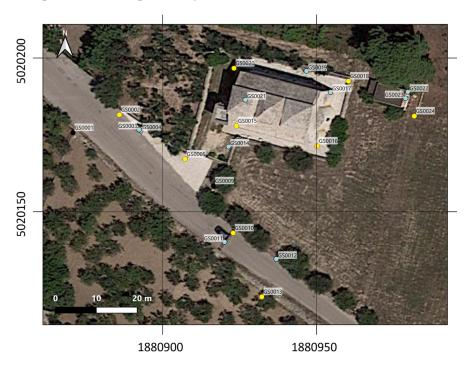
**Figure 3.** Study area: All Saints' Monastery of Cuti, located in the province of Bari (Southern Italy). The RGB orthophoto and the 3D scene representation produced by handling RPAS-photogrammetric data are reported on the left and on the right of the panel, respectively. Ground Control Points (GCPs) (in yellow) and Check Point (in light blue) locations are represented on the orthophoto. (Coordinate Reference System: WGS84/Pseudo-Mercator (EPSG:3857)).
