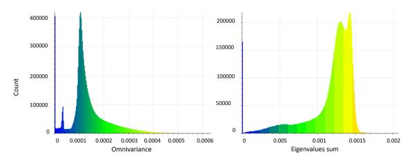
Figure 8. Histogram of eigenvalues-based geometric features extracted from the RPAS dense point cloud.
