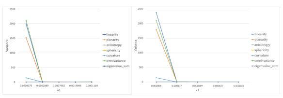
Figure 12. The variance of geometric features computed from the RPAS (on the (left)) and TLS (on the (right)) models.
