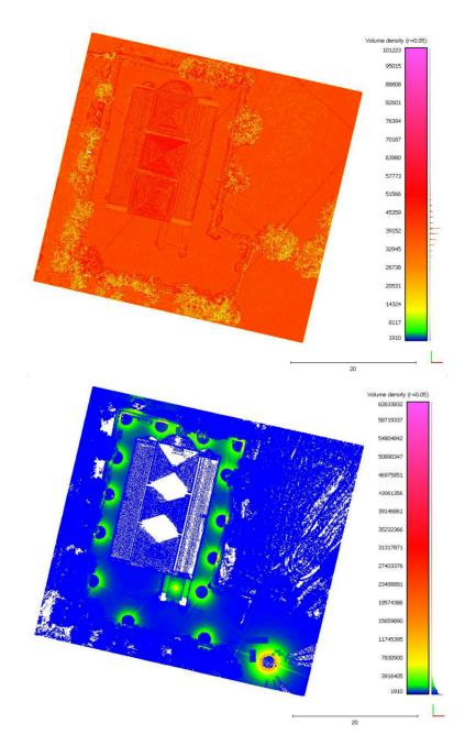
**Figure 4.** Volume density levels generated from RPAS-based and TLS-based point clouds are reported on the (**top**) and on the (**bottom**), respectively. This parameter was computed within a sphere with a radius equal to 0.05 m.
