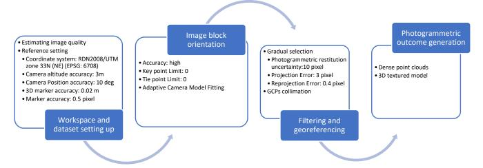
Figure 2. Photogrammetric pipeline.
