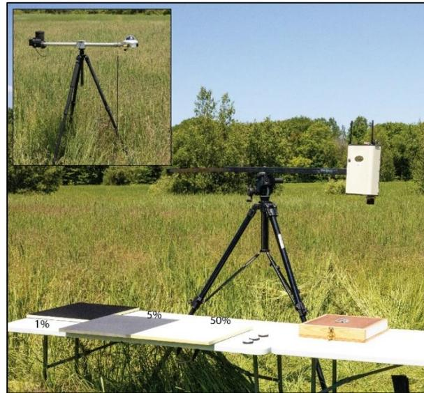
**Figure 7.** Nominal reflectance targets used for assessing radiometric quality of HSI data (VS-620). Inset shows SPN1 pyranometer and camera for hemispherical sky photos.
