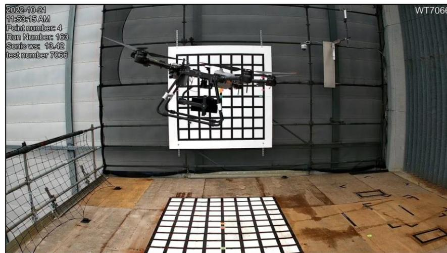
**Figure 10.** Side-view photograph of the T30 in a stationary hover at the wind tunnel exit at a wind speed of 13.42 m/s.
