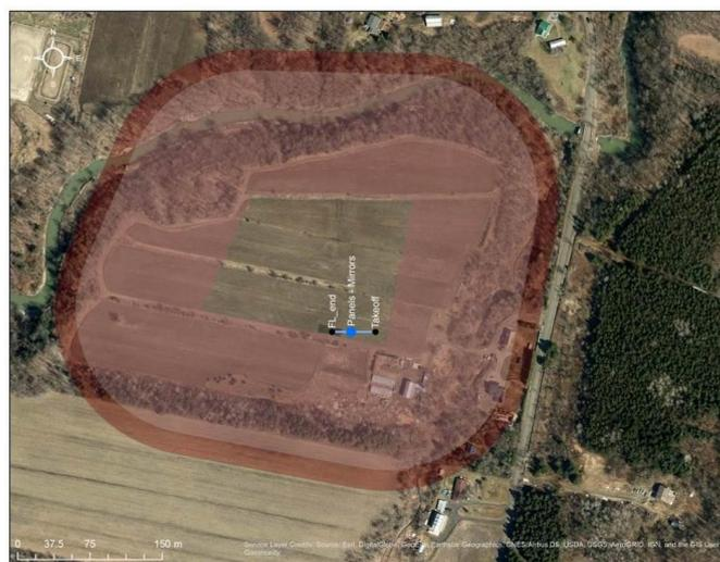
**Figure 5.** Flight line and the 500 ft and 428 ft (100 ft + maximum altitude buffer) controlled ground buffers at the Rigaud test site, Quebec.
