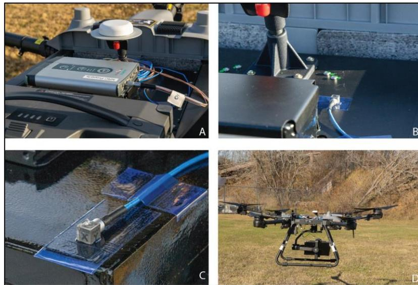
**Figure 3.** Photographs of the vibration test setup: (A) data recorder unit, (B) sensor placed on top of payload plate, (C) one of the sensors placed on the S-620 replica, (D) T30 and S-620 replica with the sensors attached during the vibration test.
