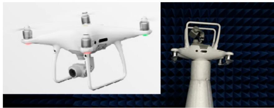
**Figure 1.** DJI Phantom 4 Pro UAV measurement environment.
