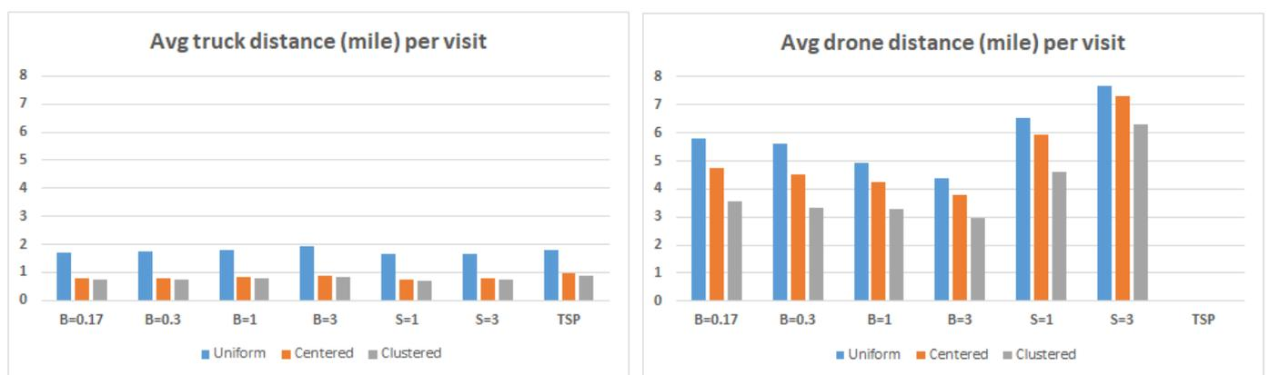
**Figure 16.** Comparison of average distance per visit traveled by the truck and the drone for 50-customer data.
