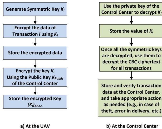
Figure 4. (a) Encryption at the UAV; (b) Decryption at the Control Center.
