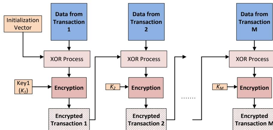
**Figure 3.** CBC process for encrypting the transaction data.
