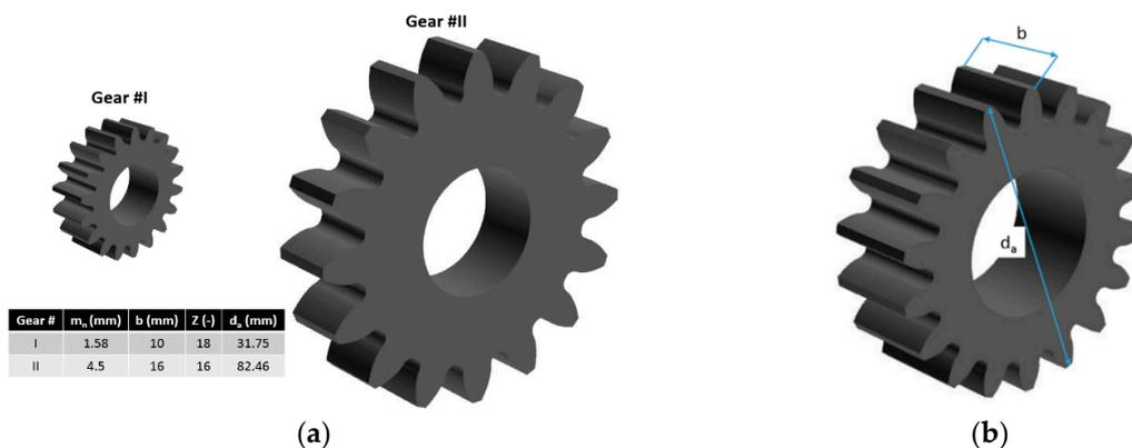
**Figure 3.** (a) The gear specification for the experiments; (b) Major dimensions of the gear considered in the analysis.
