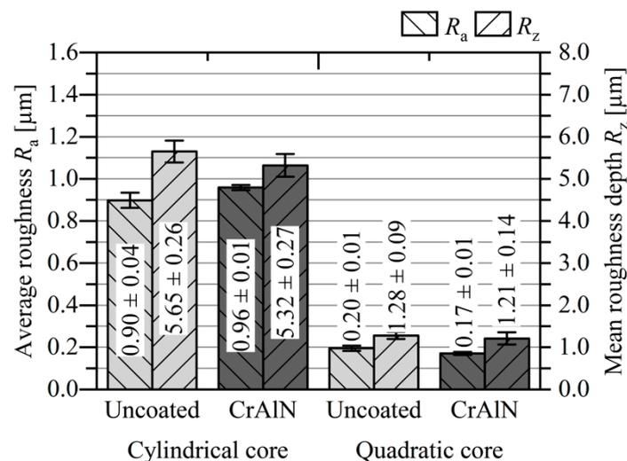
Figure 12. Average mean roughness  $R_a$  and mean roughness depth  $R_z$  of uncoated and post-treated CrAlN coated cores.
