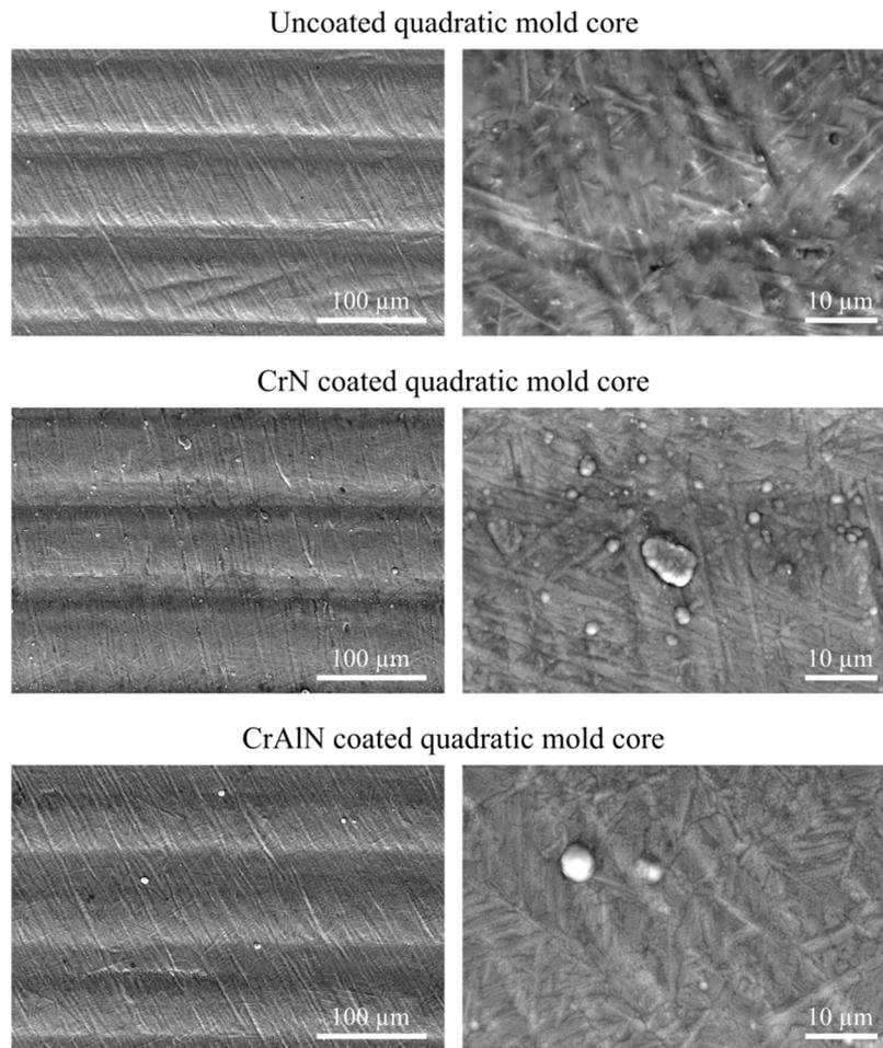
**Figure 7.** SEM micrographs of the core's surfaces with a quadratic geometry.
