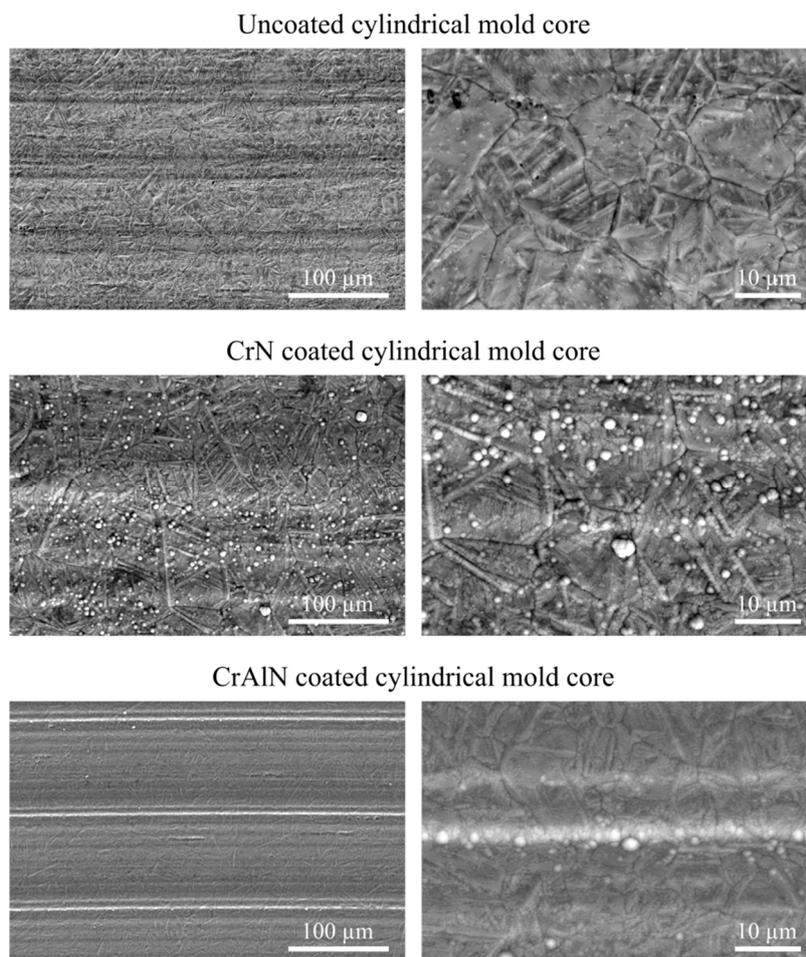
**Figure 6.** SEM micrographs of the core's surfaces with a cylindrical geometry.
