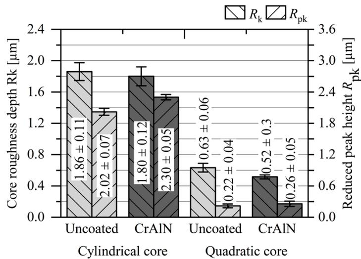
**Figure 13.** Core roughness depth  $R_k$  and reduced peak height  $R_{pk}$  of uncoated and post-treated CrAIN coated cores.
