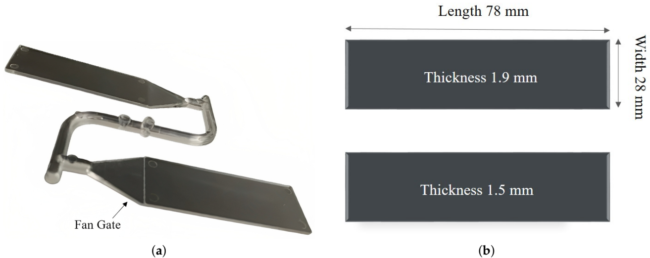
Figure 2. A schematic and dimensions of the injection molded part. Every part contains a set of two chips with two different thicknesses but which are identical in other dimensions. The chips are cut to obtain two blank slides from each part. (a) Chips before cutting the runner system; (b) Sketch of the two chips after cutting the runner system.
