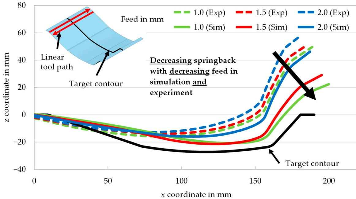
Figure 8. Comparison of springback between experimental and numerical results for varying feed with linear tool paths.
