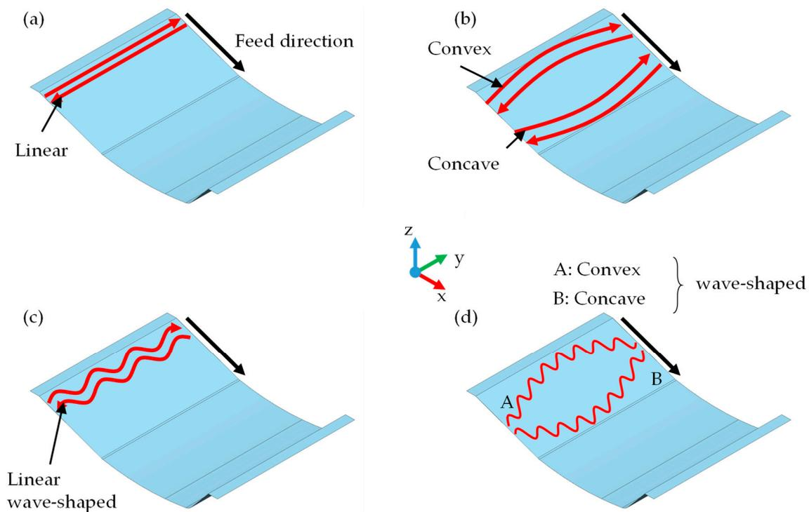
**Figure 5.** Schematic overview of tool path strategies: (a) linear tool path, (b) convex and concave curved tool path, (c) linear wave-shaped tool path, (d) convex and concave wave-shaped tool path.
