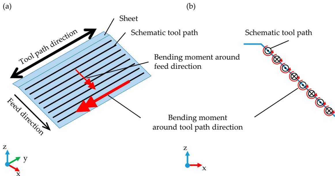
**Figure 1.** Schematic illustration of residual bending moments around the tool path direction and the feed direction in ISO view (a) and side view (b), derived from [4].
