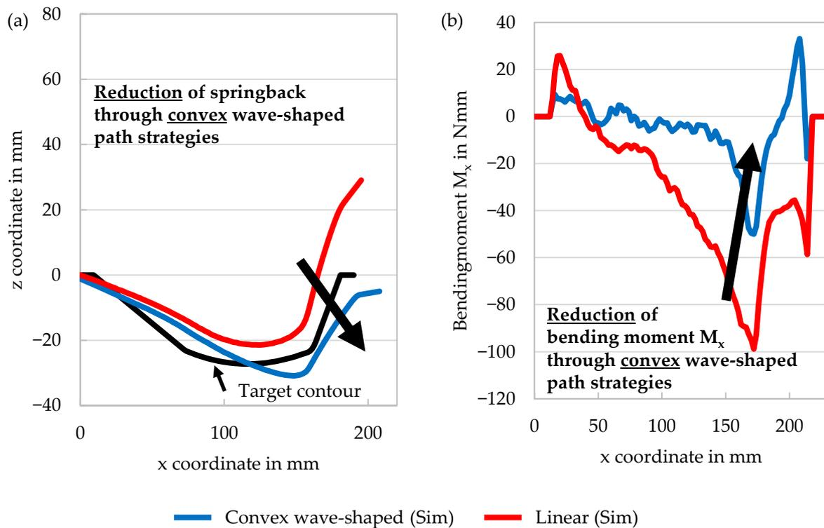
**Figure 16.** Comparison of two tool path strategies: (a) influence of the path strategy on the springback and (b) the resulting bending moment  $M_x$  before springback.
