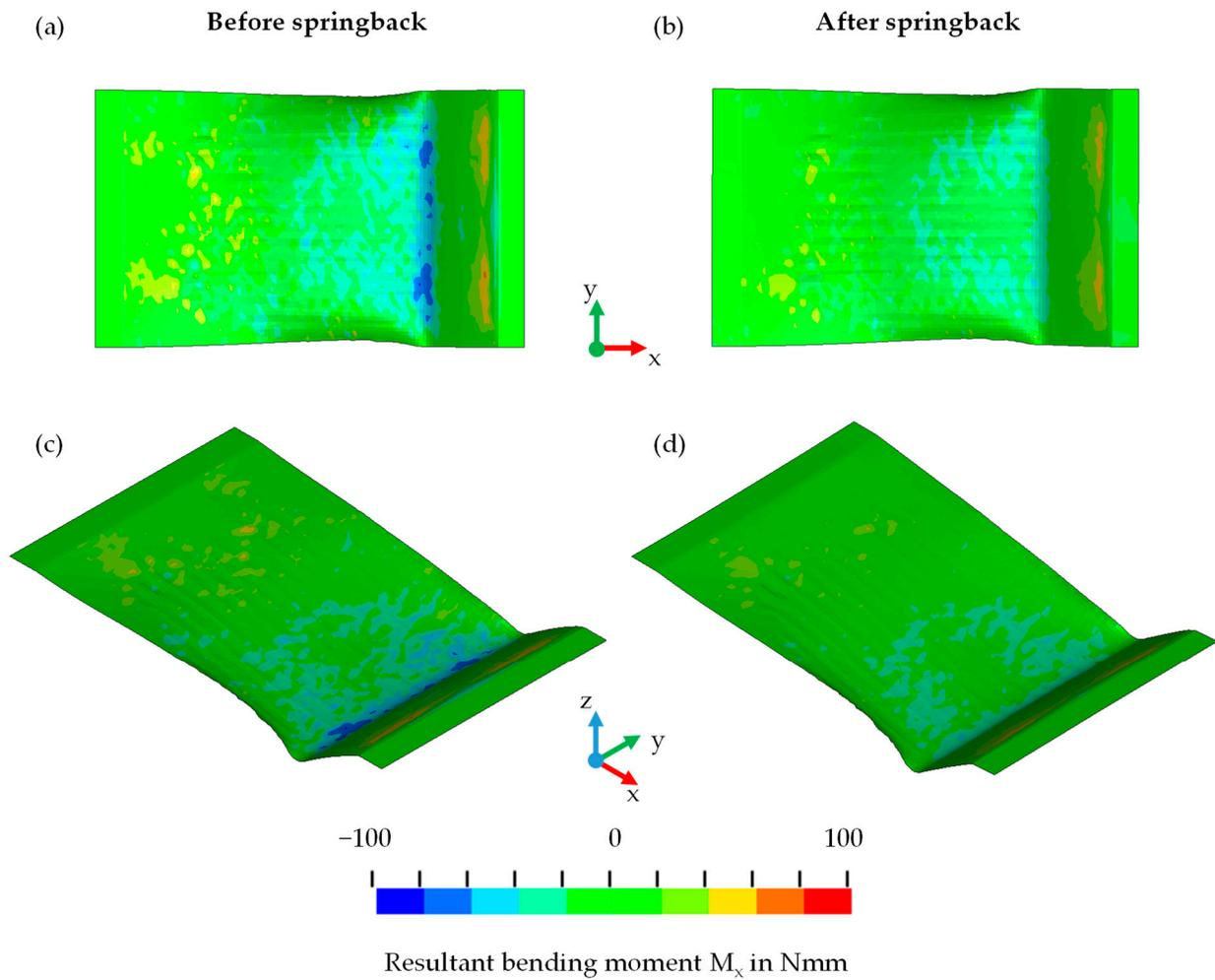
**Figure 13.** Resulting bending moments  $M_x$  for an exemplary convex wave-shaped tool path in top-view (a,b) and ISO view (c,d), before springback (a,c), and after springback (b,d).
