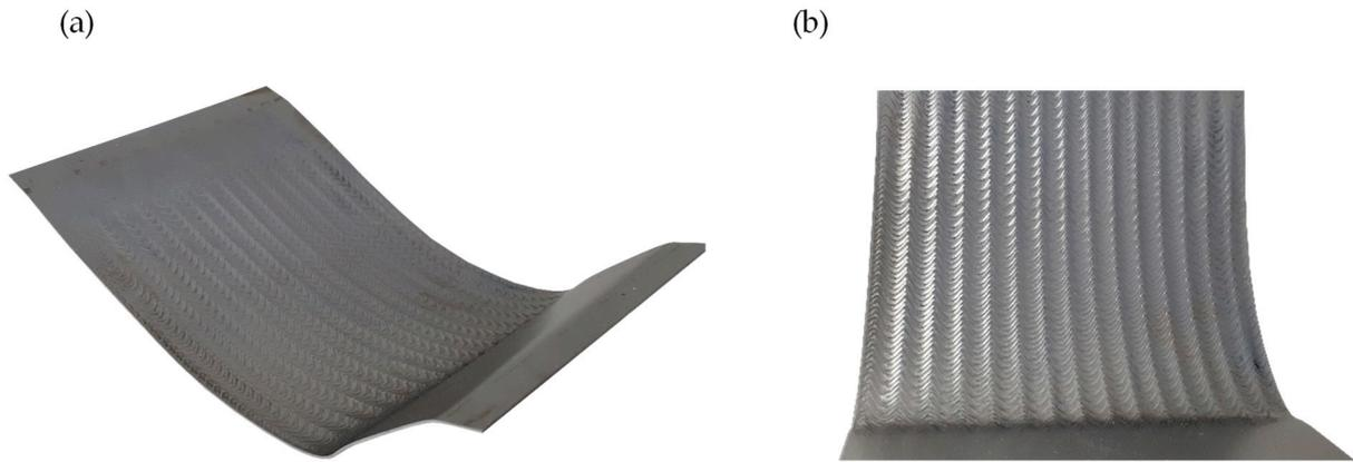
**Figure 10.** (a) Side view and (b) top view of samples formed by wave-shaped tool path strategy.
