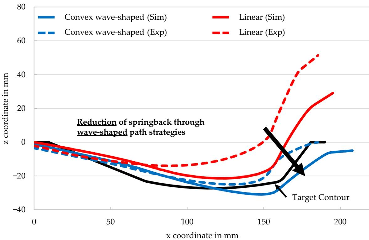
Figure 15. Influence of the path strategy on springback in simulation and experiment showing the same improvement tendency.
