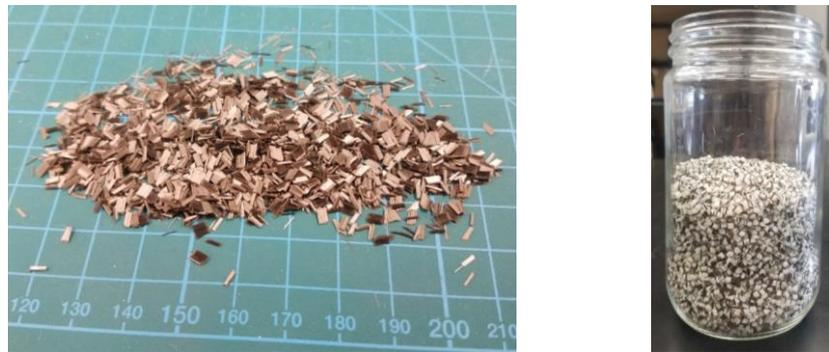
**Figure 1.** (Left) Dreytek 3 mm basalt fibers, (Right) Basalt fibers and ABS pellets premixed for compounding.
