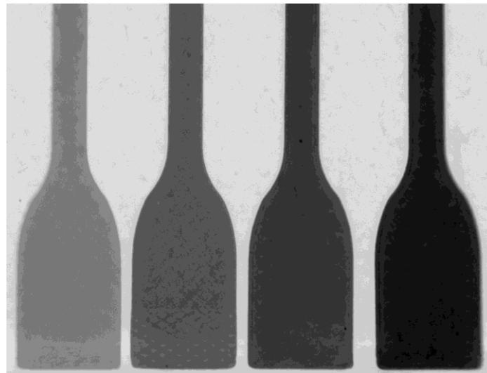
**Figure 10.** X-ray image of tensile samples with various basalt composition. From left to right: 0%, 10%, 25%, 40%.
