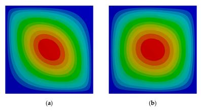
**Figure 5.** Transverse deflection surface for the optimal layups for the SSSS case. (a) constant stiffness (CS) and (b) VS.
