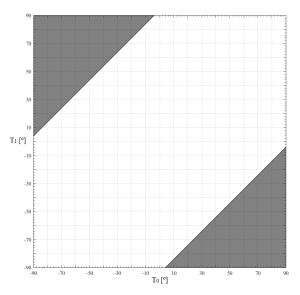
Figure 2. Feasible manufacturing fiber angles domain, in white.
