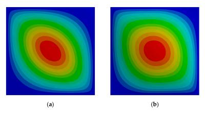
Figure 6. Fundamental vibration mode shape for the optimal layups for the SSSS plate. (a) CS and (b) VS.
