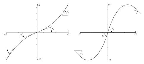
**Figure 1.** Fiber Path for  $\langle 20|60 \rangle$  configuration (**left**) and  $\langle 50|-20 \rangle$  configuration (**right**).
