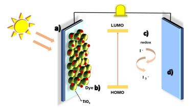
Figure 1. Typical components of a DSSC and functional mechanisms.
