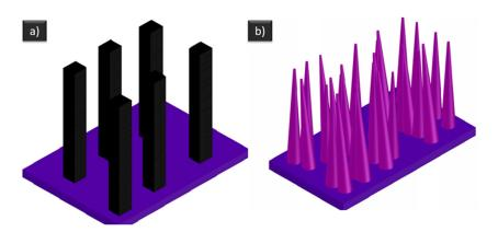
Figure 4. Schematic models of nanostructures reported in the literature: (a) nanorods and (b) nanocones.
