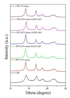
**Figure 5.** The X-ray diffraction patterns of polypropylene, mica/polypropylene and graphene oxide/mica/polypropylene films.
