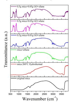
**Figure 3.** Fourier transform infrared (FTIR) spectra of mica and mica/graphene oxide before and after functionalization with silane.
