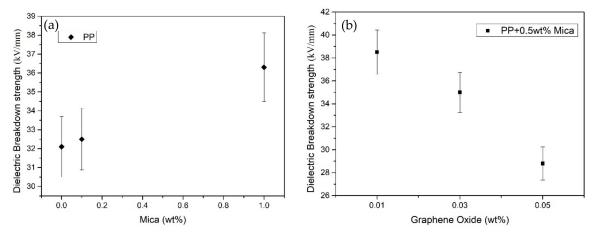
**Figure 9.** Dielectric strength comparison of all samples (**a**) the PP film with different proportions of mica addition, (**b**) 0.5 wt% mica with varying proportions of graphene oxide added to the polypropylene.
