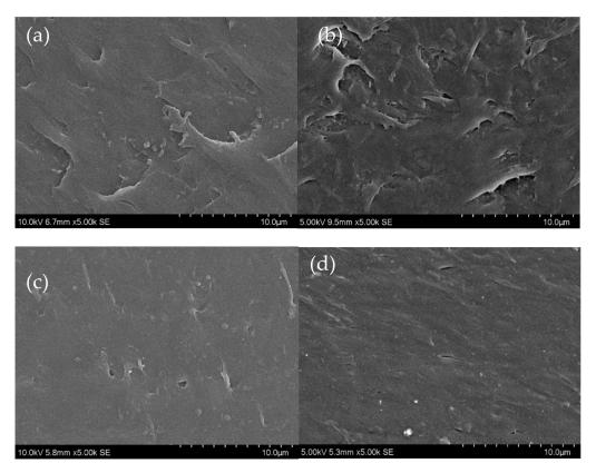
**Figure 6.** (a) The surface of the 0.1 wt% mica/polypropylene composite, (b) the surface of the 1 wt% mica/polypropylene composite (c) 0.5 wt% mica/0.01 wt% graphene oxide (GO)/polypropylene (PP) and (d) 0.5 wt% mica/0.05 wt% GO/PP SEM observation.
