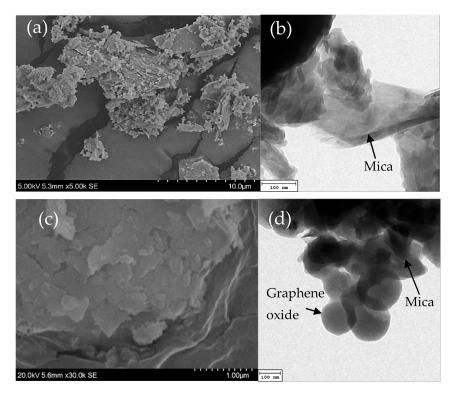
**Figure 2.** (a) Scanning electron microscopy (SEM) image of mica after microwave process (b) transmission electron microscopy (TEM) image of mica after the centrifugal procedure (c) SEM image of silane-functionalized mica platelet (d) TEM image of silane-functionalized mica/graphene oxide platelet.
