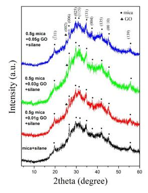
Figure 4. X-ray diffraction (XRD) patterns of silane-functionalized mica and mica/graphene oxide.
