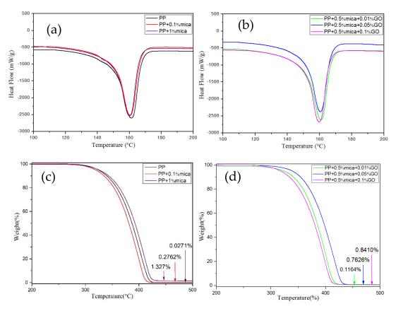
**Figure 7.** Differential scanning calorimetry (DSC) heating curves of (**a**) polypropylene (PP) and the PP/mica composites. (**b**) PP/mica/graphene oxide composites. And Thermogravimetric analysis (TGA) curves of (**c**) polypropylene (PP) and the PP/mica composites. (**d**) PP/mica/graphene oxide composites.
