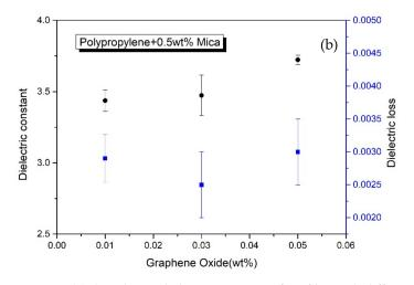
**Figure 8.** (a) the relative dielectric constant of PP film with different proportions of mica addition, (b) shows the relative dielectric constant and dielectric loss of 0.5 wt% mica with varying proportions of graphene oxide added to the PP matrix.
