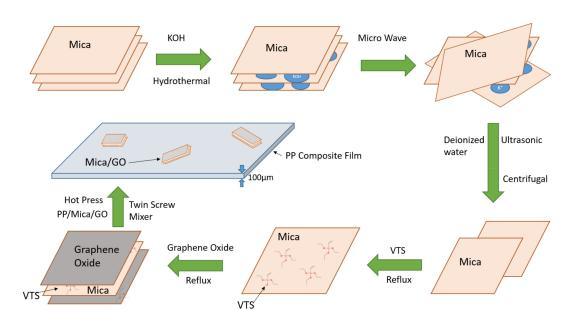
Figure 1. Mica/graphene oxide/polypropylene composite production process.
