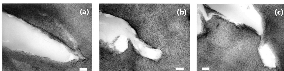
Figure 12. TEM images (osmium tetroxide stain) of ultrathin sections of MCC/MAPP/PP (22.5/2.5/75 w/w ) ternary composites with the following: (a) MAPP04, (b) MAPP12, and (c) MAPP20. Scale bars denote 100 nm. Reprinted from Ref. [33]. Copyright Elsevier Ltd. (2019).
