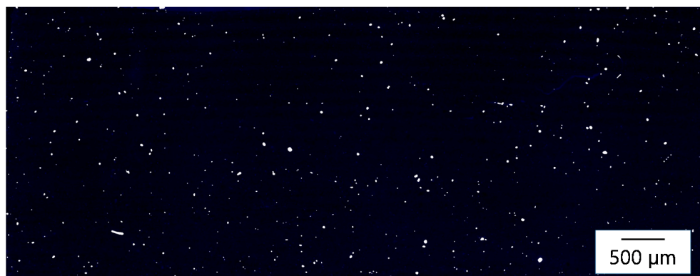
Figure 18. Typical fluorescence image (binarized) obtained by staining the cut surface of a CACNF/MAPP/PP composite (10/5/85 by weight) with CW. Reprinted with some modifications from Ref. [42]. Copyright Elsevier Ltd. (2020).
