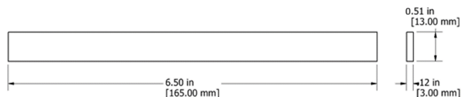
Figure 1. Rectangular coupon dimensions.
