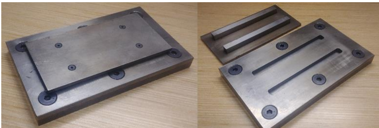
Figure 3. Mold used in the consolidation process (capable of holding two specimens simultaneously).
