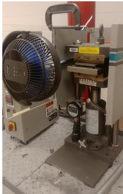
Figure 4. Hot press with electric fan setup used in consolidation process of laminates.
