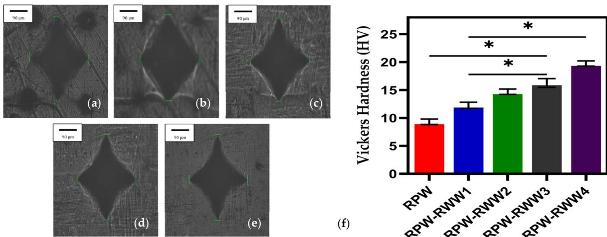
**Figure 7.** Optical micrograph images of Vickers microhardness indentation on (a) RPW; (b) RPW-RWW1; (c) RPW-RWW2; (d) RPW-RWW3; (e) RPW-RWW4; (f) Vickers hardness number of RPW-RWW composites ( $n = 3$ , \*  $p \leq 0.05$ ).
