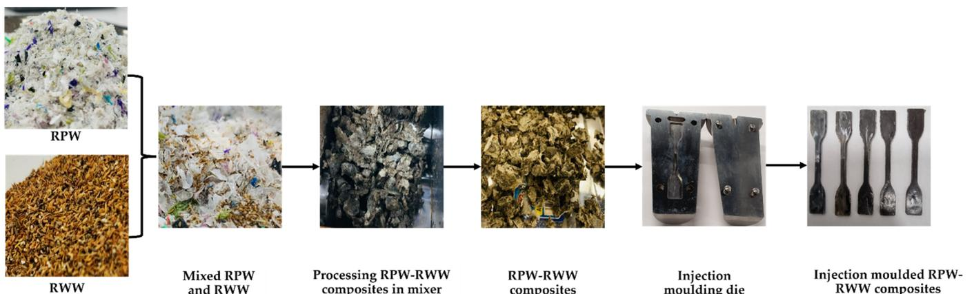
**Figure 1.** Illustration of the production RPW-RWW composites.
