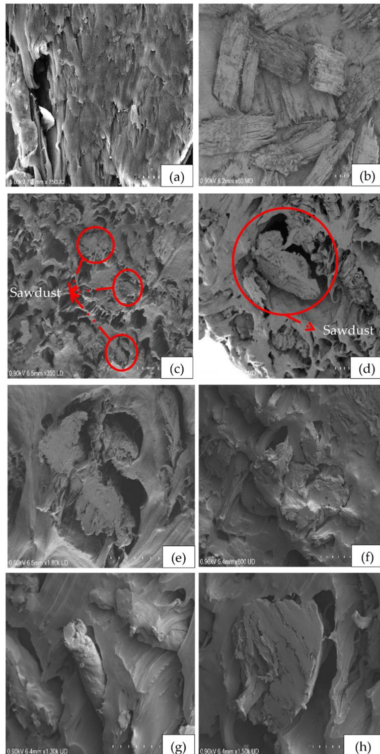
**Figure 3.** SEM micrographs (a) RPW; (b) RWW; (c) low magnification RPW-RWW4; (d) high magnification RPW-RWW4; (e–h) RPW-RWW4 cross-sectional images at different positions.
