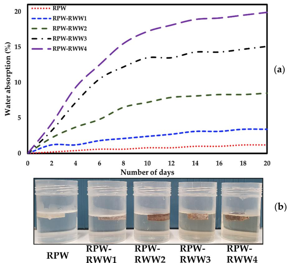
Figure 8. (a) Water absorption curves of RPW–RWW composites; (b) immersed RPW–RWW composites.
