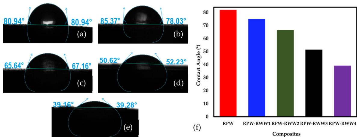
**Figure 9.** Contact angle and sessile drop images of (a) RPW; (b) RPW-RWW1; (c) RPW-RWW2; (d) RPW-RWW3; (e) RPW-RWW4; (f) Contact angle values of RPW-RWW composites.
