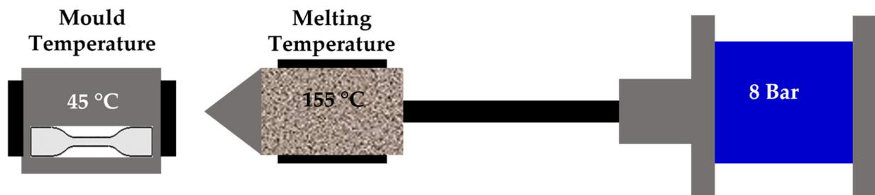
**Figure 2.** Illustration of injection moulding process.
