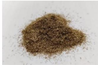
**Figure 1.** Picture of the brass fibres.
