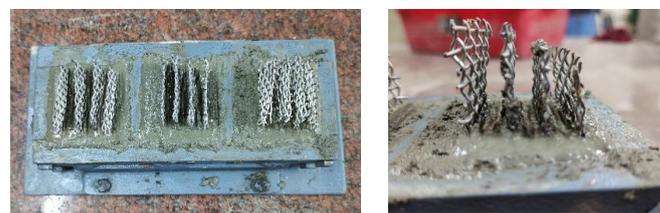
**Figure 4.** Hybrid fibre added mortar cube specimen placed with steel mesh.
