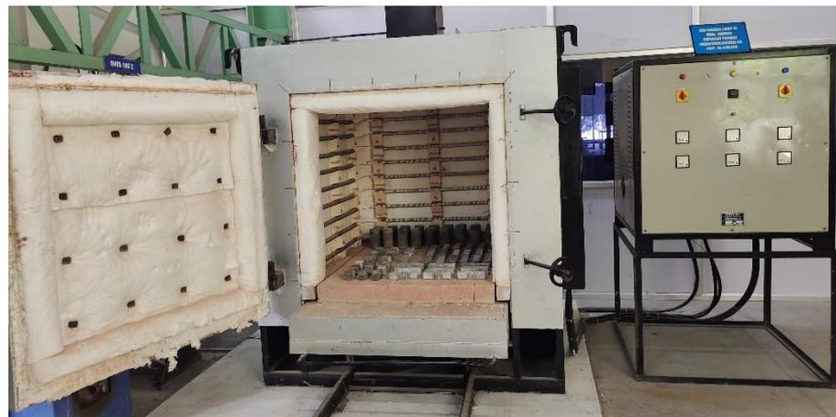
Figure 13. Specimens placed in the box furnace.
