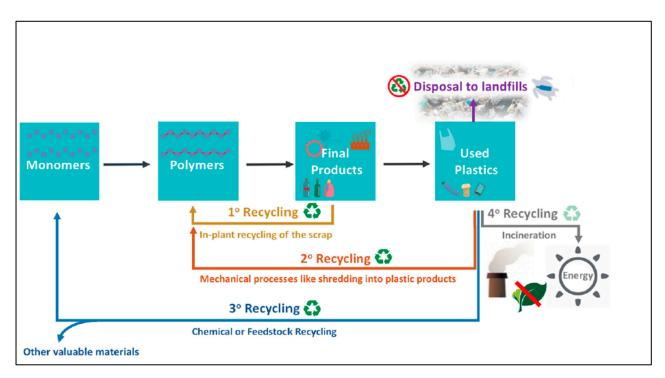
Figure 7. The four mechanisms of recycling [38].
