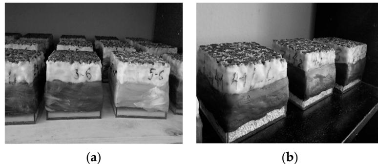
**Figure 2.** Composite specimens during the experiment with (a)  $\text{KNO}_3$  aqueous solution; (b) dry  $\text{CaCl}_2$  salt.
