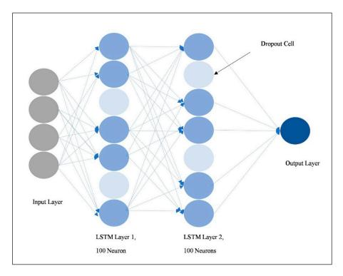
Figure 4. LSTM Network with Dropout Cells.
