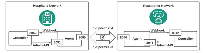
Figure 3. Networking communication architecture.
