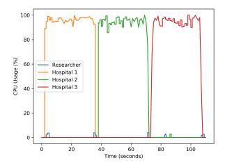
**Figure 5.** CPU Usage comparison of Docker containers during workflow using our novel federated learning libraries.
